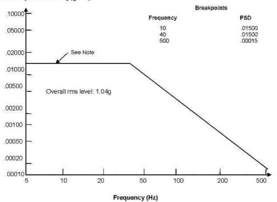
NOTE: If the item is resonant below 10 Hz, extend the curve to the lowest resonant frequency
