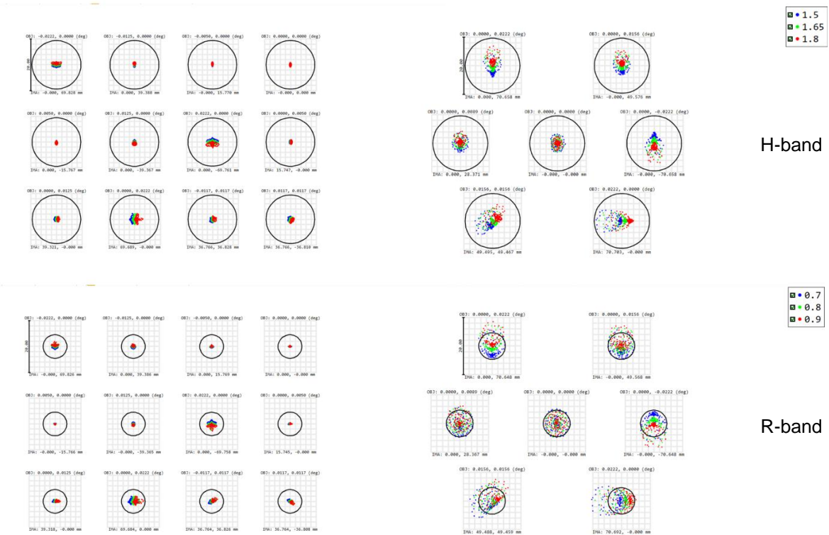
Figure 14. NGS spot diagrams comparison between the two PUA designs: new design (left) and preliminary design (right).
