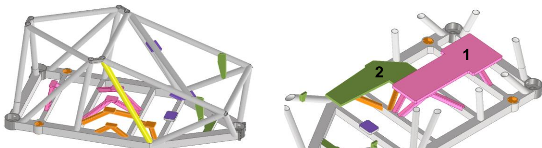
Figure 30. PUA mechanical concept: main frame on the left (the yellow beam shall be dismountable) and supporting structures on the right (highlighted in pink and green, respectively).
