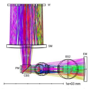
Figure 1. PUA optical layout front view (YZ plane).
