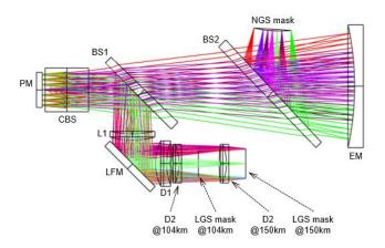
Figure 2. PUA optical layout top view (XY plane): only components positioned below W and SM.
