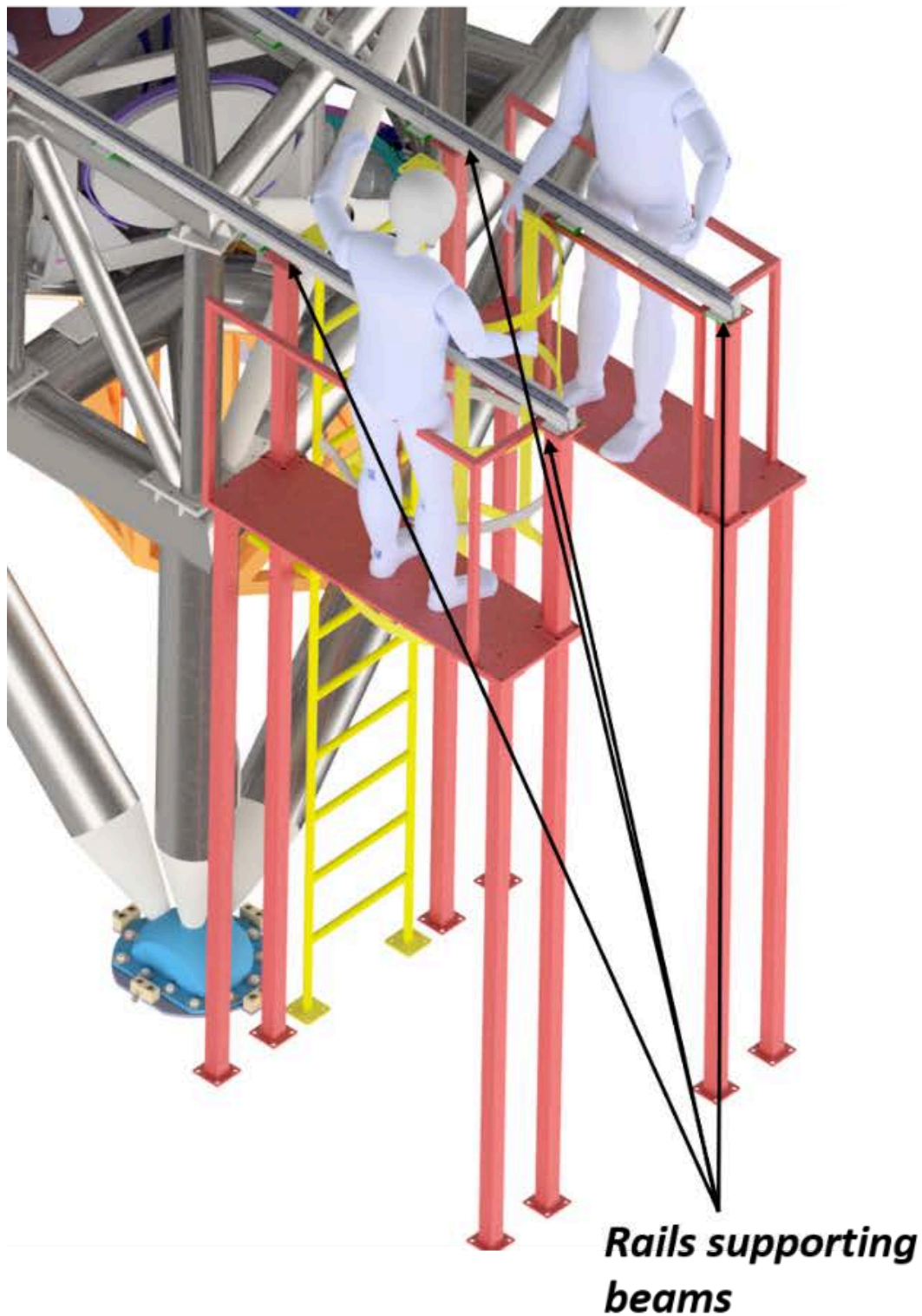
Figure 42: a view of a possible concept for the CU ladder and platforms
