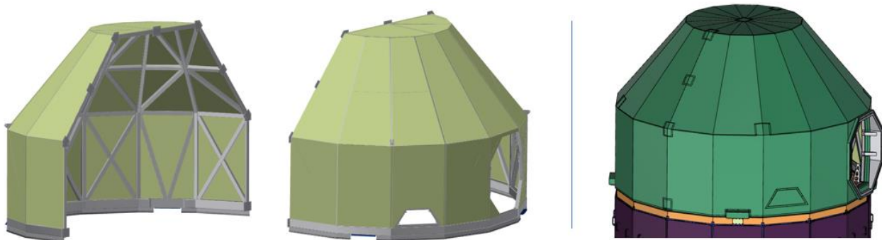
Figure 11. 3D views of MICADO Thermal Enclosure.
