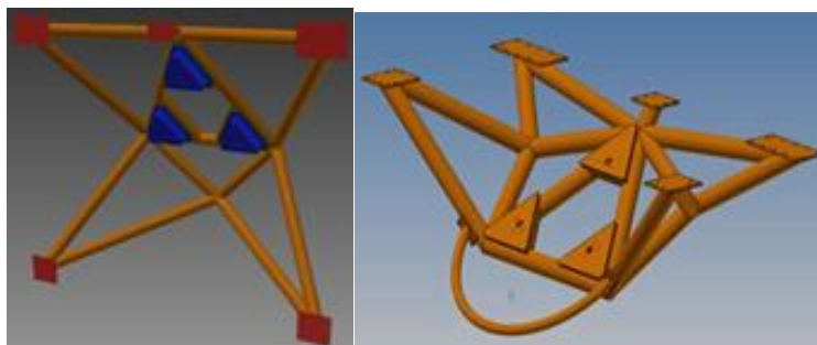
Figure 11 : Optomechanical Support Structures of M8 (left side) and M7 (right side).
