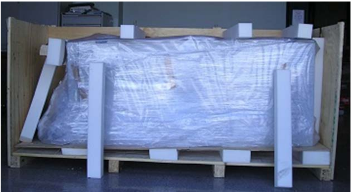
Figure 3: Floating packing for electronic cabinets
