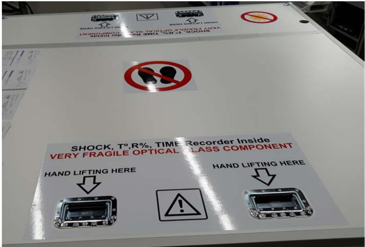
Figure 8: Example of inserted handles.
